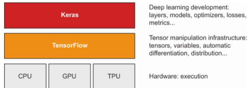
Figure 3.1 Keras and TensorFlow: TensorFlow is a low-level tensor computing platform, and Keras is a high-level deep learning API
